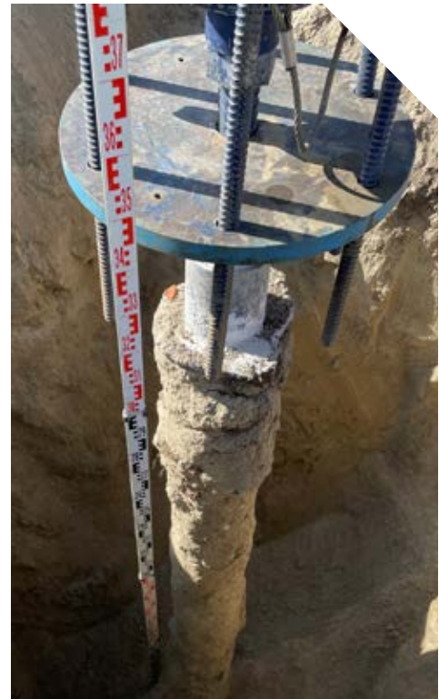
TEST PILE PP02 EXPOSED to a depth of approx. 3.2m
